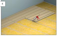
Forestia Thermofloors are installed offset to each other. The panels must be pressed so tightly together that adhesive emerges from the joints. Remove excess adhesive.
