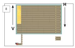
The right side is installed from top to bottom, while the left side is installed from bottom to top. This is to ensure that the panel's profile fits.
