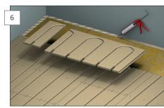
Cut and adjust the first Forestia Thermo Turn Board. Apply chipboard adhesive to subfloor or joists. Make sure that the return groove is placed over the joist. The inner radius of the return groove must be at least 10 mm in on the joist. There must be a minimum 10 mm expansion gap between Thermofloor and Thermo Turn Board.
