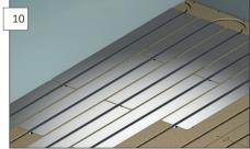
Before pressing the heat diffusion panels into place, all grooves must be carefully cleaned of adhesive, debris and other impurities. Any peaks or raised edges at joints must be levelled off by grinding. There should be 10 mm clearance between the heat diffusion panels. Terminate the panels 10 mm before the start of the return on the Thermo Turn Board.
