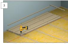
Against all fixed structures there must be a clearance of 10 mm. Cut the first panel. Clean the profile on the short side of the Thermofloor that is to lie against the straight edge of the Forestia Thermo Turn Board. We recommend installing Forestia Thermofloor before installing the Forestia Thermo Turn Board. Use 4 screws at each panel end and 4 screws for each joist. Use chipboard screws of dim. 4.2x55 mm or equivalent.
