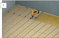
Make sure that the grooves in the Forestia Thermo Turn Board are aligned with the grooves in the Thermofloor. Use 6 screws at each panel end and 4 screws for each joist. Use chipboard screws of dim. 4.2x55 mm or equivalent.
