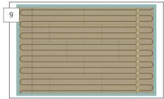
Forestia Thermofloor and Thermo Turn Board are fully assembled. The Thermo Turn Board is pre-drilled with holes for incoming and outgoing pipes. Ensure that there are no sharp edges when inserting and extracting pipes. This is to avoid damage to underfloor heating pipes.
